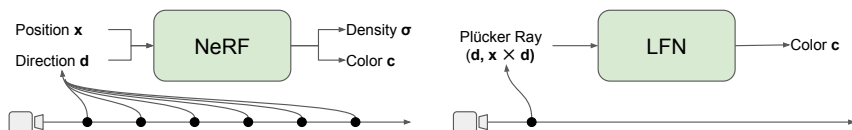
Figure 2: LFNs directly predict the RGB color for each ray in a single inference using Plücker coordinates, avoiding the dozens to hundreds of inferences required by NeRFs.
