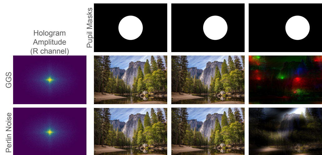
Figure 15. Eyebox comparison between GGS and Instant-SFH with Perlin-noise-based phase at 80% sparsity. The pupil mask (top row) shows the pupil moving progressively to the right. The center row shows images reconstructed from GGS. The bottom row shows images reconstructed from Instant-SFH using Perlin noise.
