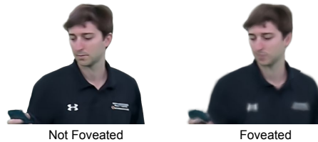
Figure 7: An example of foveated rendering from our progressive multi-scale LFN. Foveated rendering generates peripheral pixels at lower levels of detail to further improve performance in eye-tracked environments. In this example, foveation is centered over the left eye of the subject.
